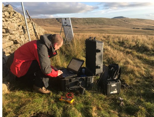
Figure 3: An example of a temporary station. Power is provided by the solar panel in the background. The sensor is buried and is not visible here.
